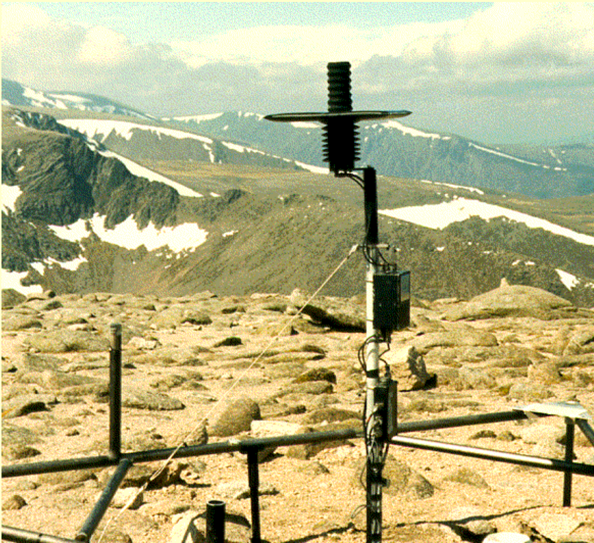
Heriot-Watt University automatic weather station, Cairngorm summit
