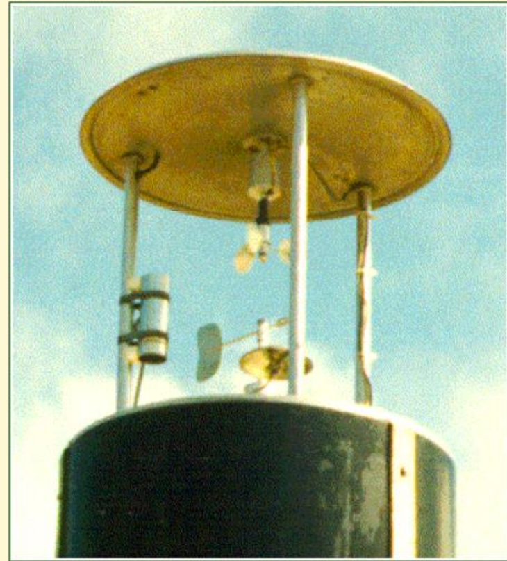
Institute of Hydrology Automatic Weather Station: instruments emerge from the protective cylinder every fifteen minutes to take readings. The rim of the cylinder is equipped with a heating ring to overcome rime and icing up in winter.
