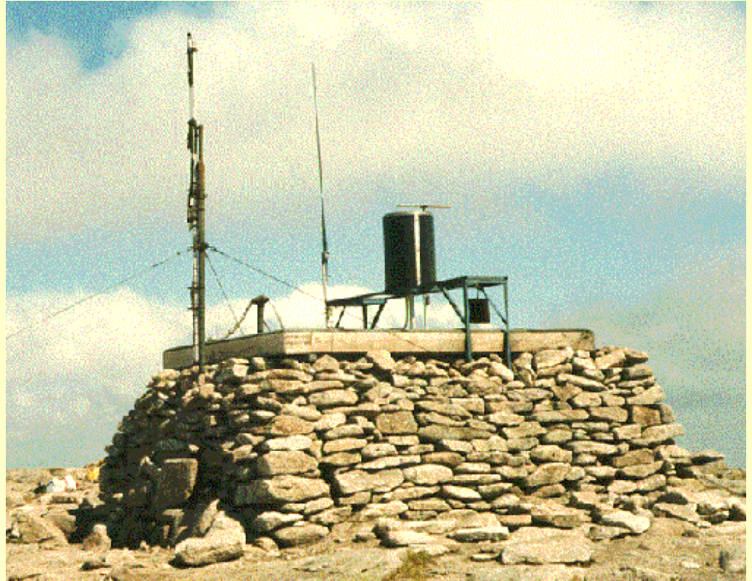
Institute of Hydrology automatic weather station, Cairngorm summit
