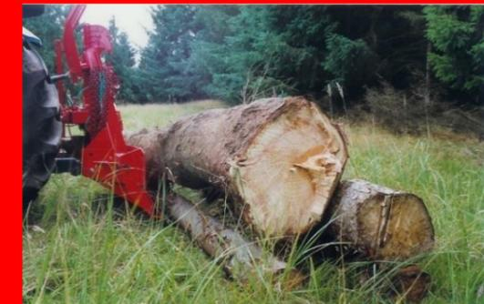
The winch can also be used for "stacking" logs and leveling
