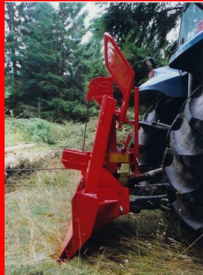
Extra support on the top pulley provides additional resistance when pulling heavier logs
