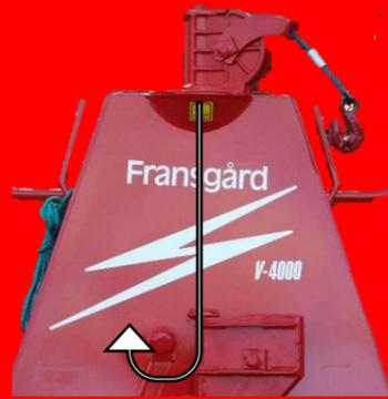
The longer distance between the top pulley and cable drum enables optimal cable spooling.
