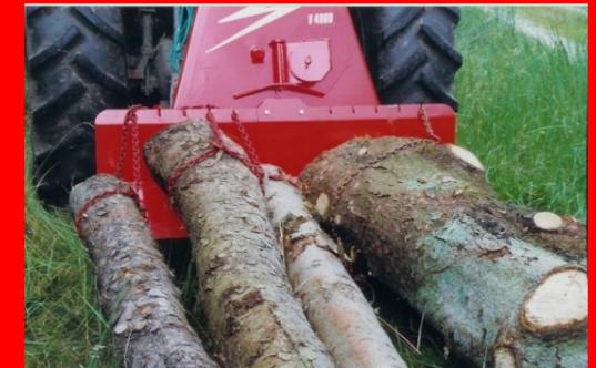
The dozerblade is designed with additional height and a wide log-towing bar to handle even the largest logs.
