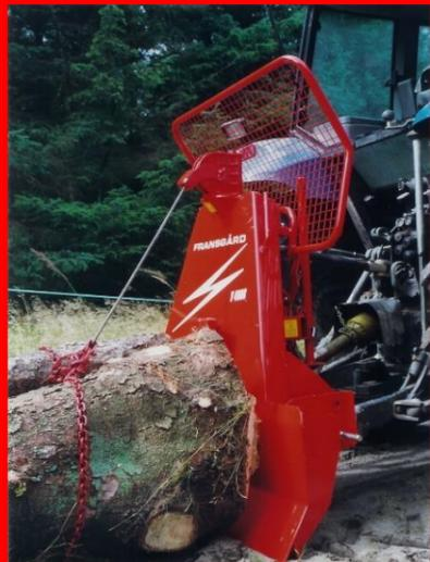
Protective screen guards the tractor in case a cable should break.
